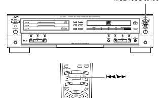
When the last track on a CD loaded in the 3-CD changer is advanced to the next track, playback moves to the first track on the next CD. It is not possible to skip forward when playing the last track of a CD loaded in the CDR.
