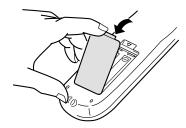
2 Place the two accompanying R6P(SUM-3)/ AA(15F) batteries in the remote control making sure to match the battery polarities with the markings ("+"/"-") inside the compartment.
